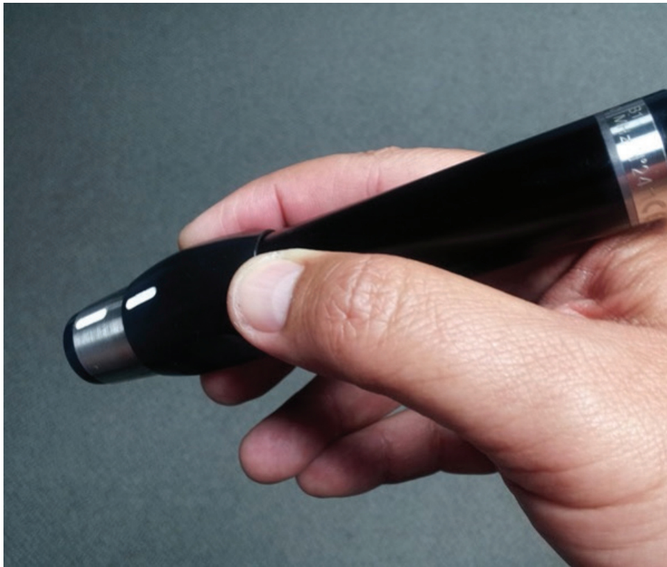
Fig 27: B-mode transducer line indicates the area shown at the top of the screen.
