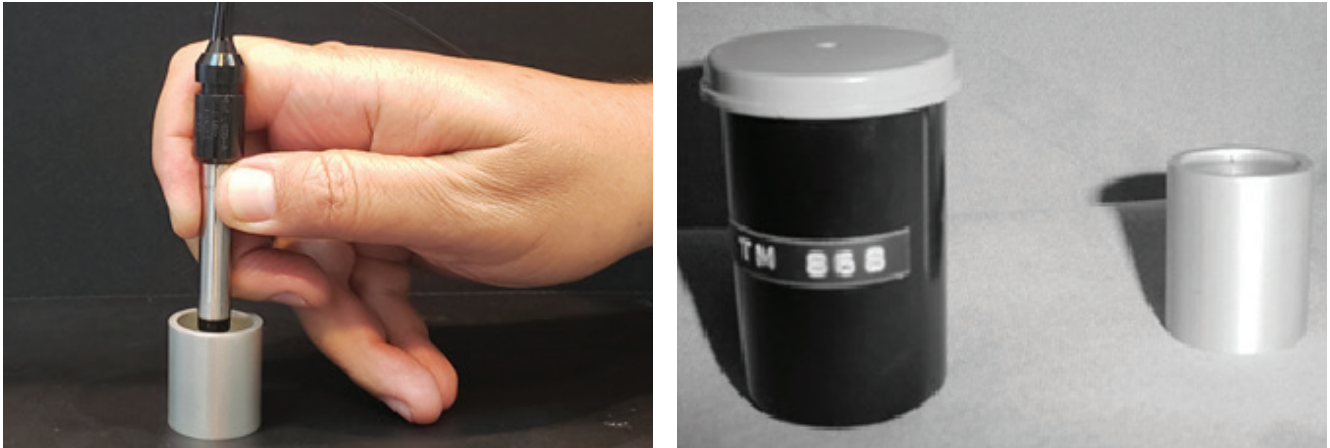
Fig 19.1: Calibration of the probe to using the tissue model (TM 868) in order to obtain tissue sensitivity.
