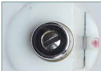
Fig.2 ► Top view of the Berens-Tolman Tonometer. The moulded plastic prism and the lines for alignment to ascertain pressure above or below normal are illustrated
