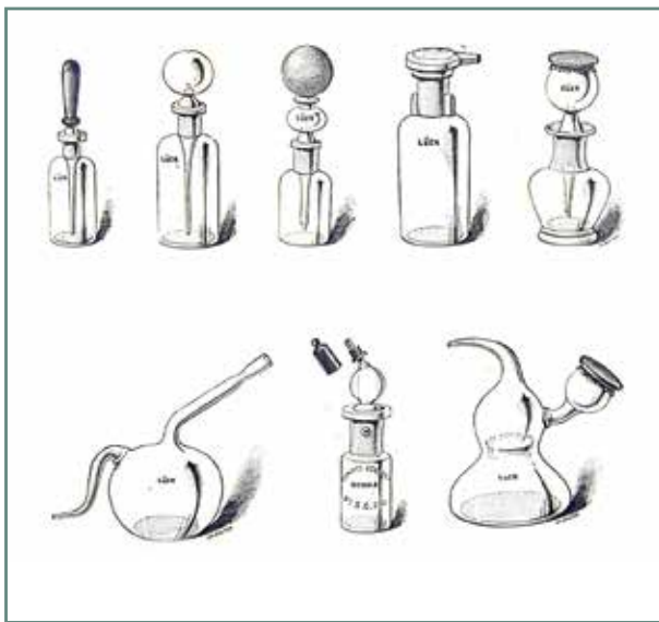
Fig.1 ▶ Undines of different shapes and sizes. The flow through the spout could be controlled by pressure on the diaphragm or blocking the opening of the straight arm with a finger tip
