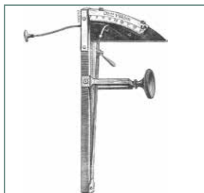
Fig.2 ► The Fick Oswald ophthalmotonometer where a smoked glass plate was incorporated to facilitate reading of the pressure value
