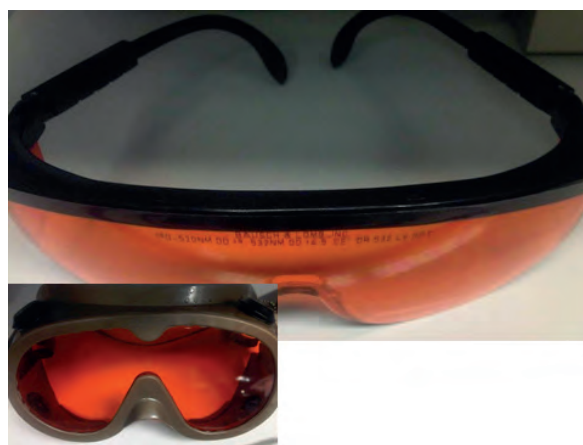
Figure 4. The goggles have a label on its lens or frame indicating the optical density for each wavelength range. Each person is responsible for confirming that the goggles are appropriated for the laser wavelength in use and has correct optical density that allows adequate ocular protection. The colors of the glasses do not confer any secure indication, only the label on the goggles can do it.
