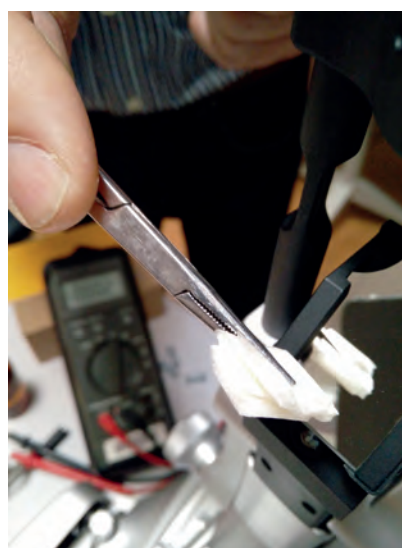
Figure 2. Example of external optical cleaning.
